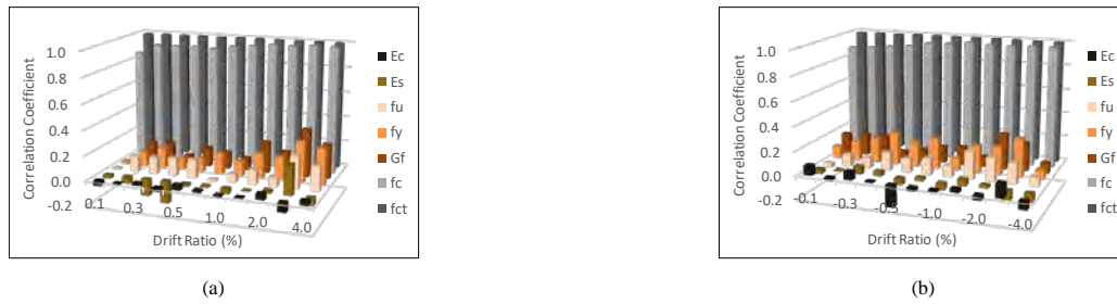
Fig. 5.7 Sensitivity analysis in the reference specimen EJ-R (a) positive loading direction (b) negative loading direction
