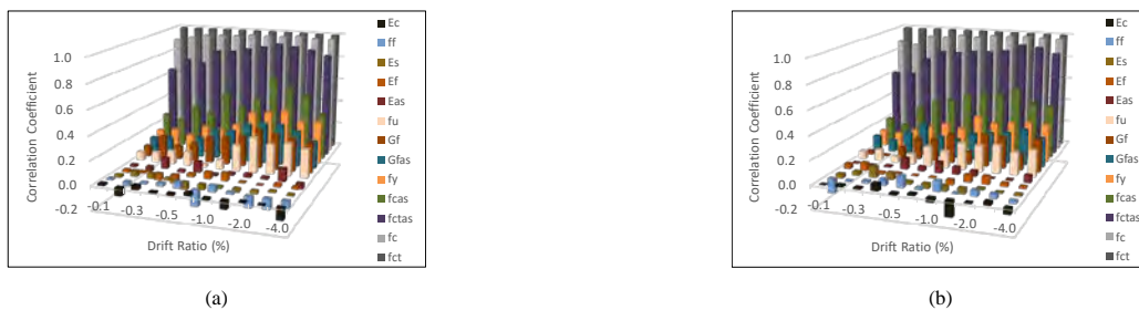
Fig. 5.8 Sensitivity analysis in the retrofitted specimen (a) positive loading direction (b) negative loading direction
