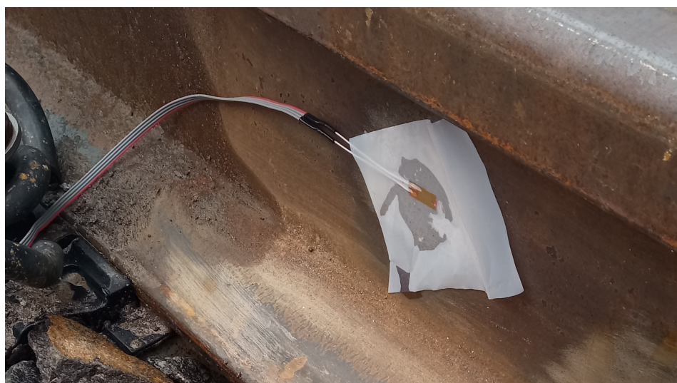
Figure 3: Strain gauge attachment by 1-70 fast-acting superglue.
