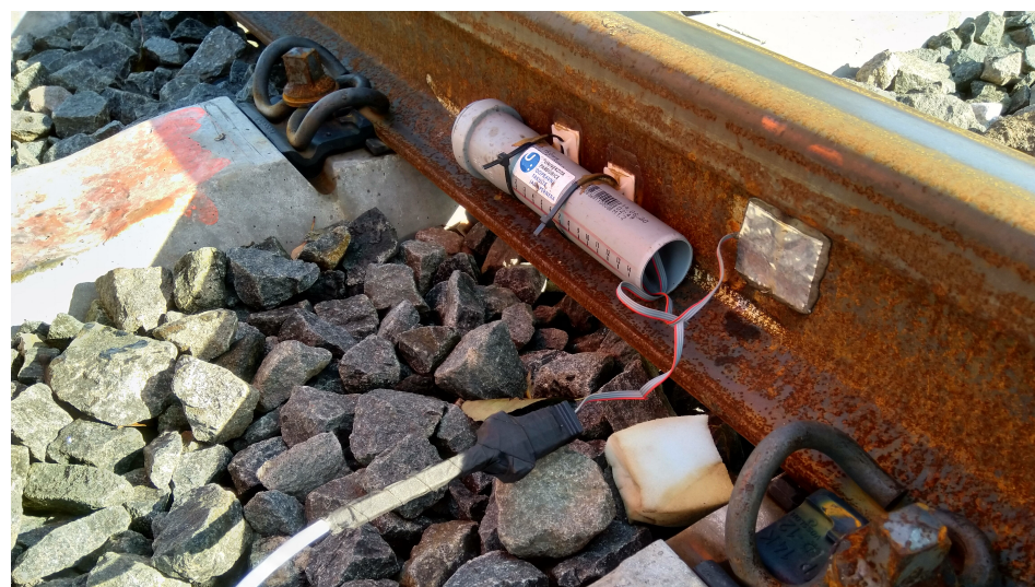
Figure 4: Connection of track and mobile part of the measuring set during measurement.
