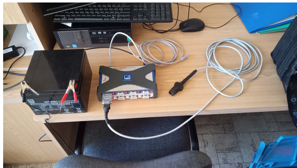
Figure 2: Mobile part of the measuring set.
