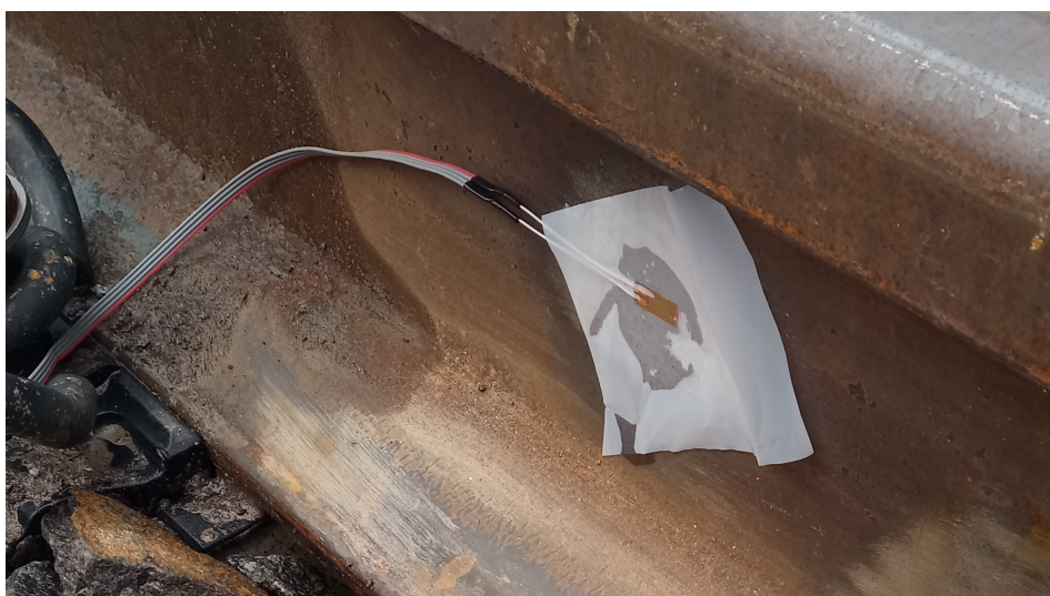
Figure 3: Strain gauge attachment by 1-70 fast-acting superglue.
