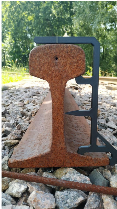
Figure 8 – 3D Printed Rail Neutral Axis Gauge.
