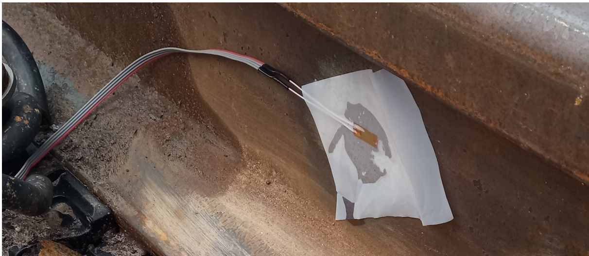
Figure 4 – Glued Strain Gauge (with Teflon Cover) with Marked Horizontal Lines.
