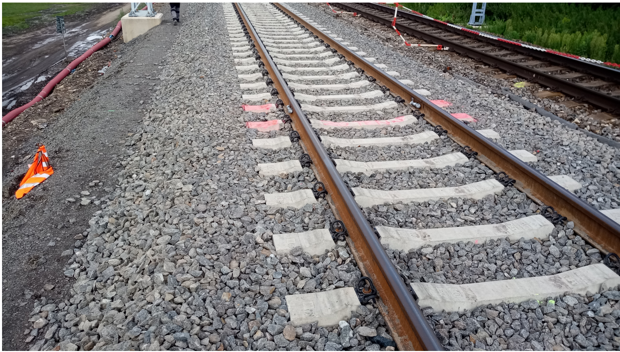
Figure 9 – Marking of Stationing with Measuring Spots in the Bezprávi Measuring Locality by Red Colour on the Upper Surface of Sleepers Outside the Track Channel and by a Flag Made from an Orange Reflective Vest.
