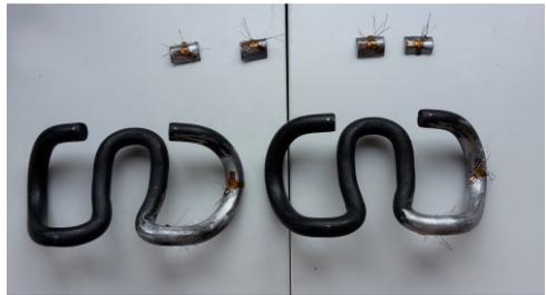
Fig. 7-6: Strain gauge location - place I
