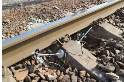
Fig. 7-11: Detail of the location of displacement sensors
