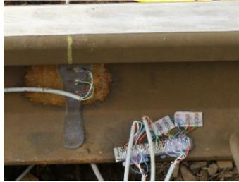
Fig. 7-9: Location of strain gauges for Y and Q measurements
