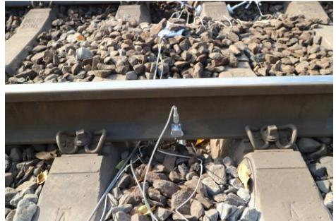
Fig. 7-15: Detail of acceleration sensor location
