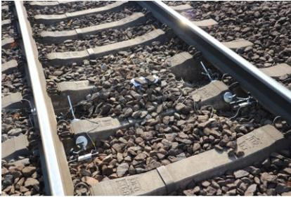
Fig. 7-10: Location of displacement sensors
