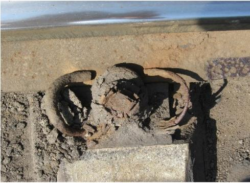
Fig. 1-1: Clamp with large corrosion loss of material
