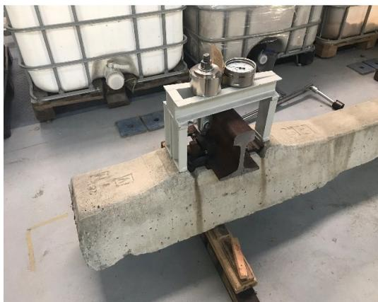
Fig. 4-6: Vossloh device for measuring of the clamping force
