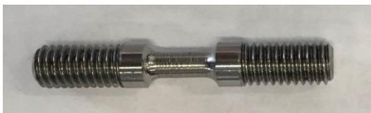
Fig. 4-1: Sample for tensile test
