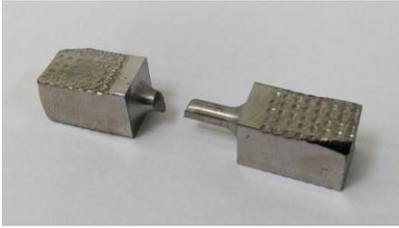
Fig. 4-3: Sample after fatigue test
