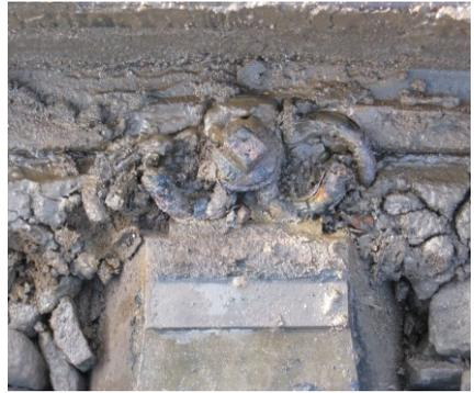
Fig. 1-2: Cracked clamp
