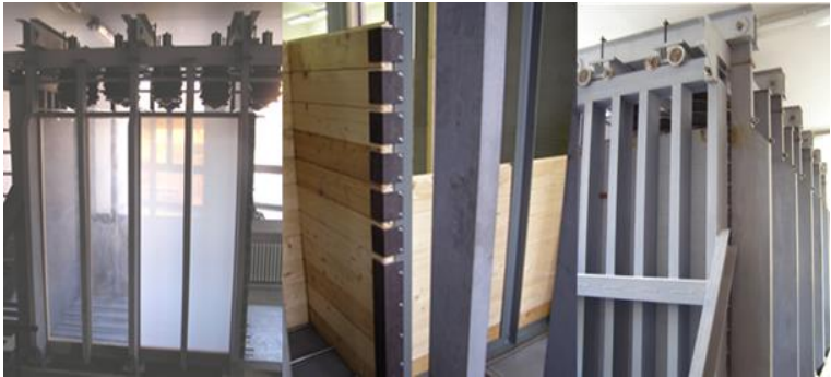
Figure 3.1. Steel Frame Used during Construction and Testing
