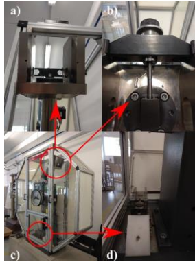
Figure 3.5 a) Pendulum hammer, b) Screwed specimen between tail block and tup, c) General view of Zwick/Roell RKP 450 pendulum impact tester and d) Anvil
