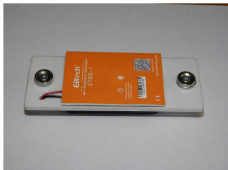
Figure 2.3 – Card Thermometer Holder – Top View
