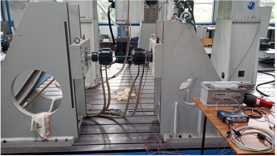
Figure 3.2 – Steel Sample Positioned in the Dynamic Stand
