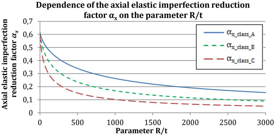
*Fig. 1: The illustration of the axial elastic imperfection reduction factor  $\alpha_x$  for three fabrication tolerance quality classes.*
