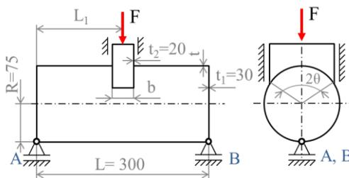
Fig. 3: The schematic of geometric parameters of a laterally loaded cylindrical shell.
