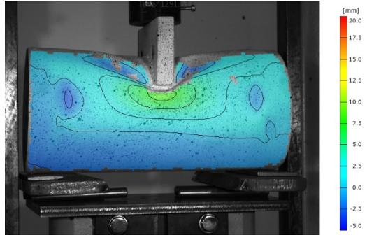
*Fig. 7: Deformed experimental model (at  $u_y\sim 10.3$  mm) - ARAMIS system.*
