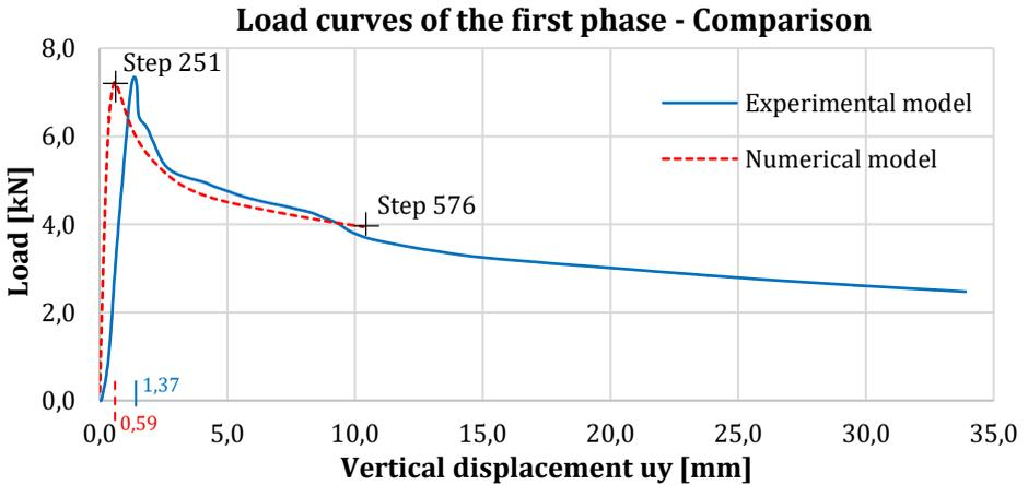
Fig. 5: Load curves – the comparison of experimental and numerical model – first phase of verification.
