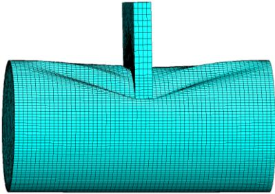
*Fig. 6: Deformed numerical model of the ideal shell at the end of loading (at  $u_y=10.33$  mm, computational step 576, 1:1).*
